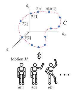
Figure 1: Robot posture, motion in the joint space
